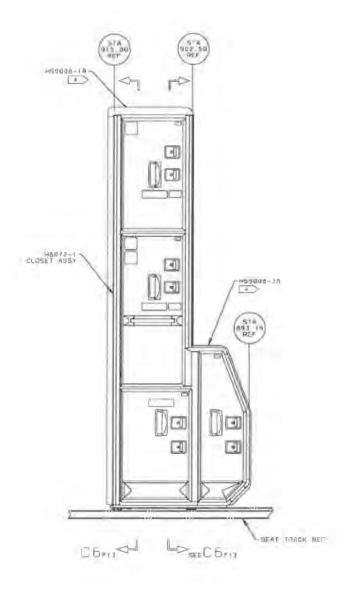
10. The Qantas B737-400 Aft LH Closet is a single integrated structure that has a contoured forward wall. The forward wall is shaped to conform to the shape of a passenger seat located immediately in front of the closet. The forward wall is specifically contoured to include a chamfer at floor level to receive passenger seat legs. The upper portion of the forward wall also is contoured to receive and conform with the shape of the passenger seat back located immediately in front of the closet.
